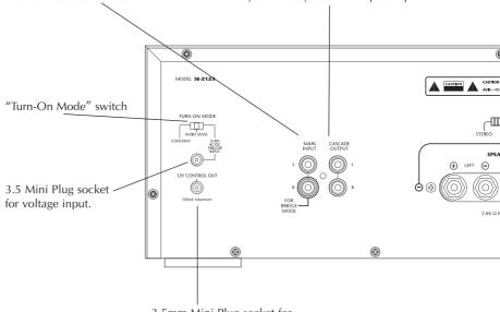
3.5mm Mini Plug socket for 12v DC Control output.
